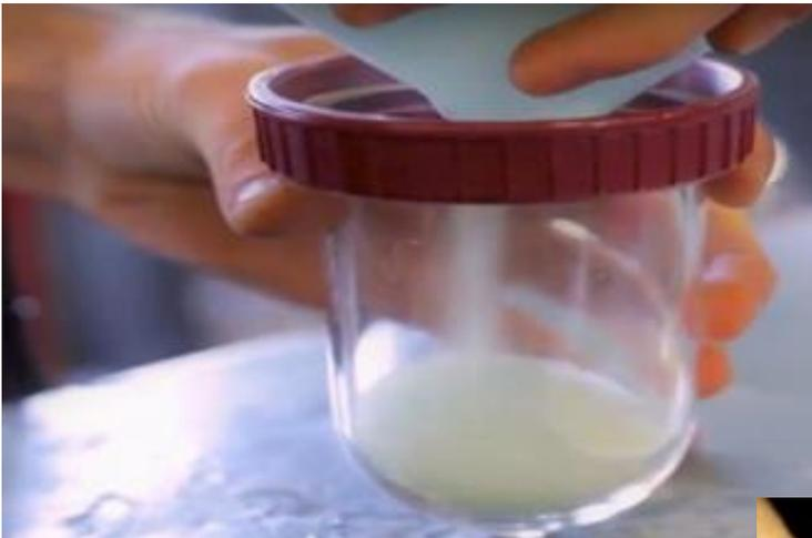
3. Fill clear reservoir with desired amount of Counteract Balancing Beads.
