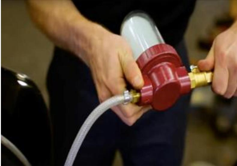
8. The injection should only take 20-40 seconds. Ensure feedline is clear. Remove clip-on chuck. Close air-valve on injection tool.
