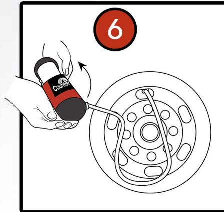
When ready, open the air valve to allow dry air into the tire and then begin to rotate the pump upright slowly. Be sure this is done gradually to allow the beads to easily flow out of the pump and into the tire. Be mindful not to over-inflate during this process. Once all the beads are in the tire, shut off the air valve and remove the chuck.
