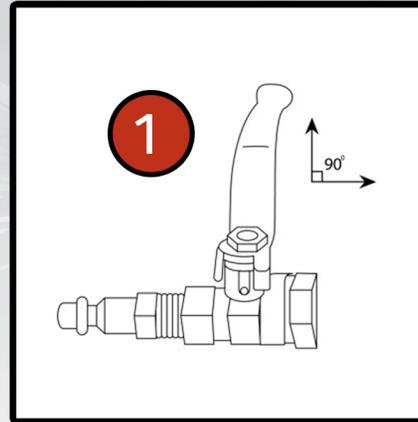
Ensure the ball valve is in the CLOSED position. The black handle must be perpendicular to the air hose connection (90 degrees)
