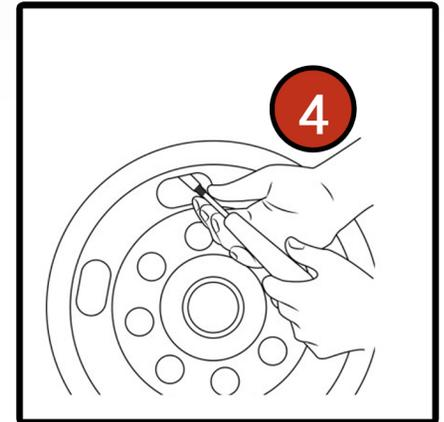
Ensure your valve is either at the 12 o'clock or 6 o'clock position. Remove valve core from the tire's valve stem. Allow tire to deflate to approximately half of its PSI. Do not deflate fully, unless the vehicle is supported by jack stands relieving any pressure from the wheel.
