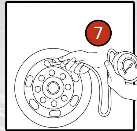
Install your valve core and torque it to the recommended 4-inch pounds. Over-torquing may damage the core causing an air leak. Proceed to air the tire up to the recommended PSI for your application.
