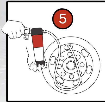
Rotate the pump so that the reservoir is pointing down (6 o'clock), ensure your valve is in the CLOSED position and connect your airline. When the tire is deflated, connect the chuck to the valve and make sure it is secure.
