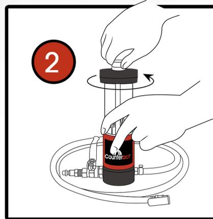
Unscrew the silver cap nut and remove the black top plate. Inspect for cracking, chips, and damages. Ensure the cap nut thread is free of cross threading and damage.
