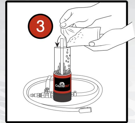
Open your desired amount of Counteract Balancing Beads and carefully pour them into the clear reservoir. Once you have finished pouring the beads, make sure none are on the edge of the reservoir, and that the thread is clear of debris. Proceed to press the black top plate on the pump and secure it with the silver cap nut. Finger tight is all that is needed.
